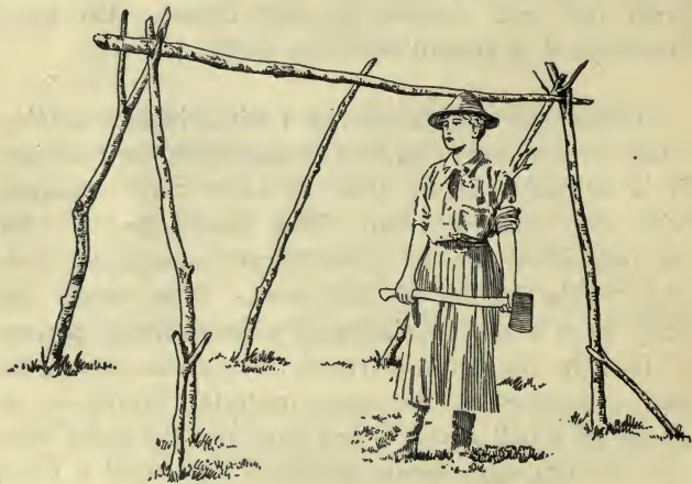
FIG. 9.—Frame for Lean-to Shelter
