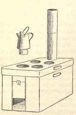
of ten to twenty. It was almost an indispensable article with such large companies. It is a round-cornered box, twenty-one inches long by twenty wide, and thirteen inches high. with a slide in the front end to admit air and fuel. The bottom is fixed to the body; the top removes, and
