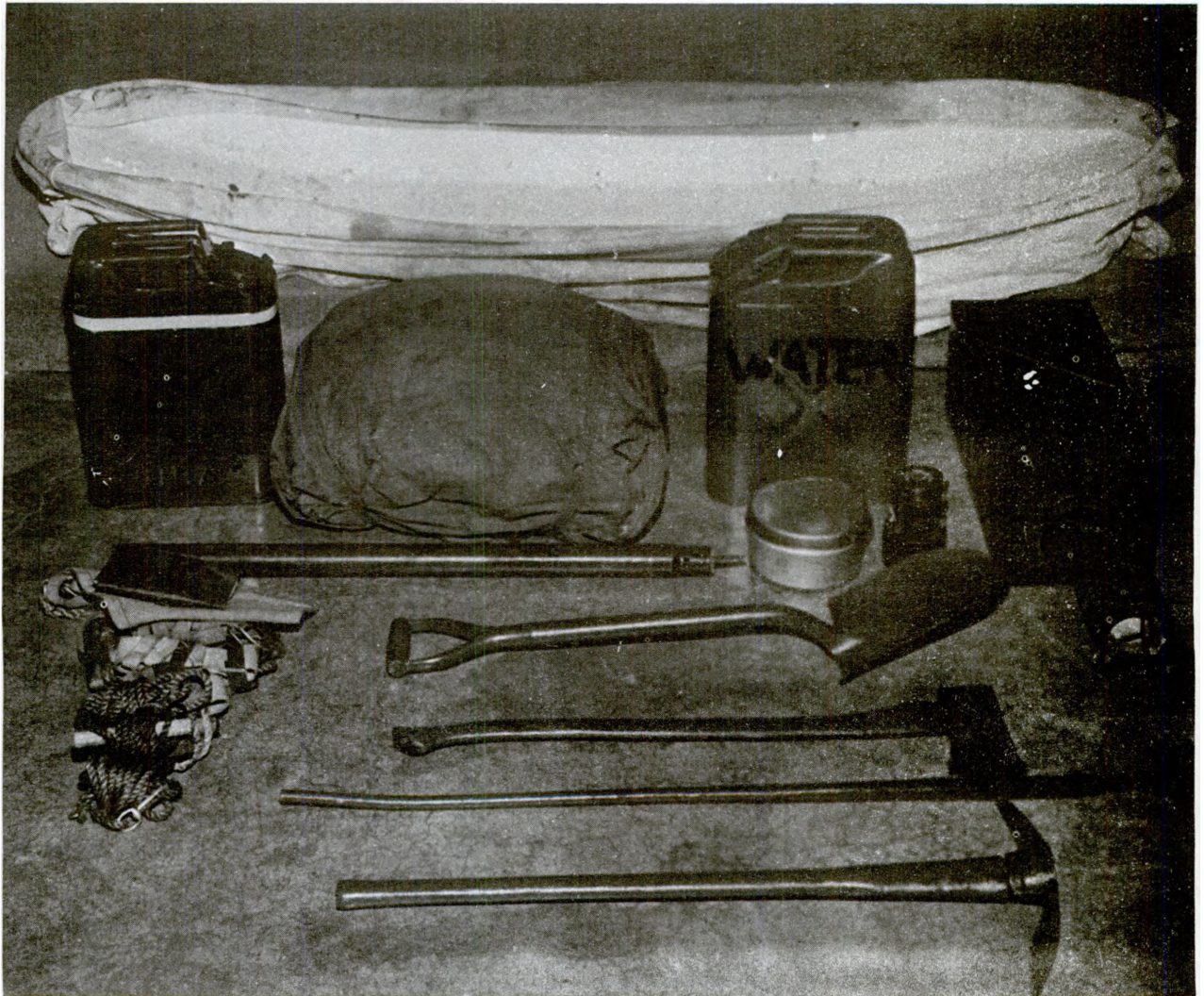
Figure 5-13. Sled, scow-type, 200-pound capacity, with tent group equipment.
