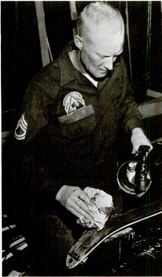
Figure 4-5. Heating pine tar with a blowtorch.
