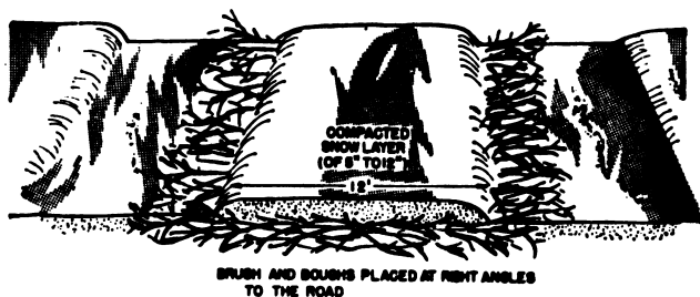
Figure 5-8. Road reinforced with brush and snow.
