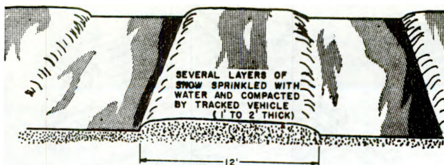
Figure 5-7. Road reinforced with snow.
