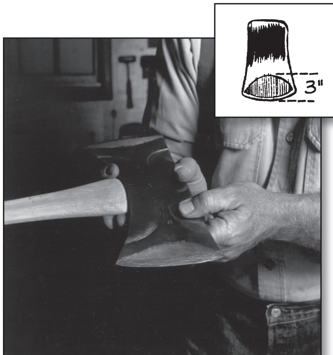
Figure 66—When sharpening, try for a fan-shaped effect on the cheek of the ax (drawing by Frederic H. Kock).
