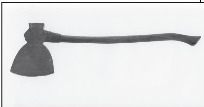
Figure 18e—A 19th-century shipwright's mast broad ax.
