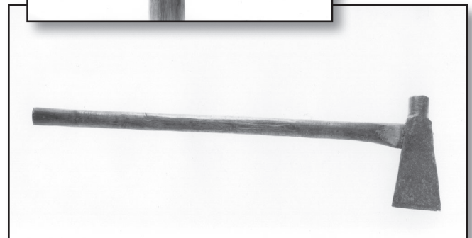
Figure 8—An 18th-century splitting ax, with straight handle typical of early axes.
