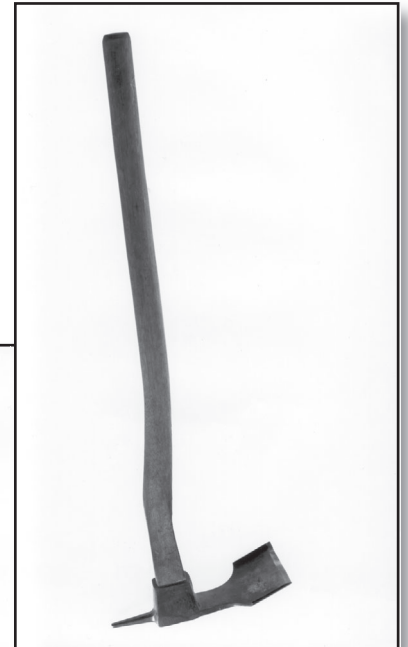
Figure 27a—Collins lipped shipwright's adz.
